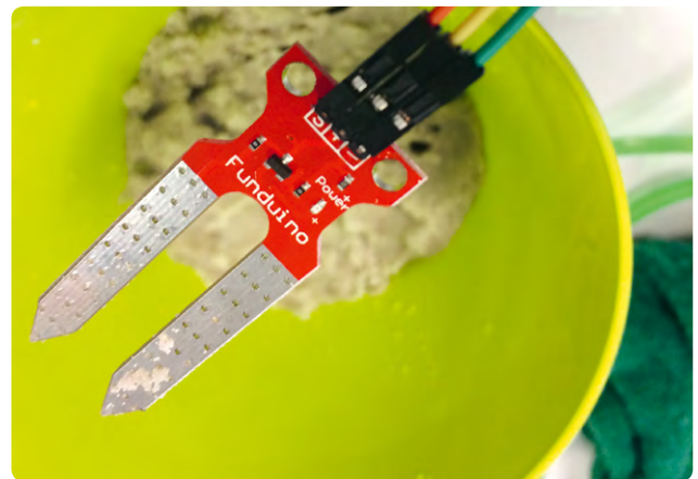
10: A soil moisture sensor
